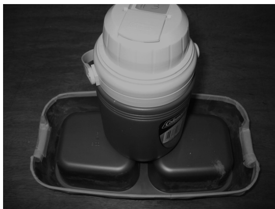
Fig. 1. A dry ice trap consisted of an inverted cat feeder and an insulated jug.
